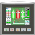
The generator is controlled using the latest in HMI touch screen technology to display the process, pressures, inlet air dewpoint and oxygen levels with continuous monitoring complete with alarms.
