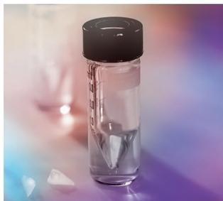
Mounted on a triangular matrix, these small Teflon-coated stirring bars fit the cone portion of 0.3, 1.0, 3.0, 5.0 and 10.0 ml Thermo Scientific Reacti-Vial Small Reaction Vials. For more information on Reacti-Vial Small Reaction Vials, see page 5.
