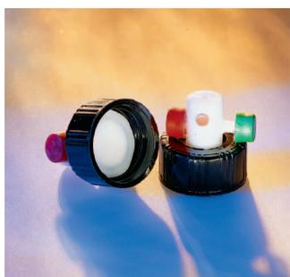
They're easy to use. Push the green button to open, insert syringe needle and take sample, withdraw needle, then push red button to close. To change needle-seal septa, simply push the old septum out with a 1/8" diameter rod and push a new cylinder septum in. This is done with the valve closed to prevent exposure of contents.
