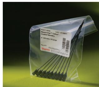
Thermo Scientific Reacti-Vap Teflon Coated Needles are made exclusively for use in Reacti-Vap Evaporators. They are blunt-ended, 19-gauge, stainless steel needles that reduce cross-contamination and corrosion when evaporating solvents that contain strong acids.
