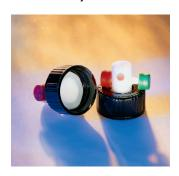
They're easy to use. Push the green button to open, insert syringe needle and take sample, withdraw needle, then push red button to close. To change needle-seal septa, simply push the old septum out with a 1/8" diameter rod and push a new cylinder septum in. This is done with the valve closed to prevent exposure of contents.
