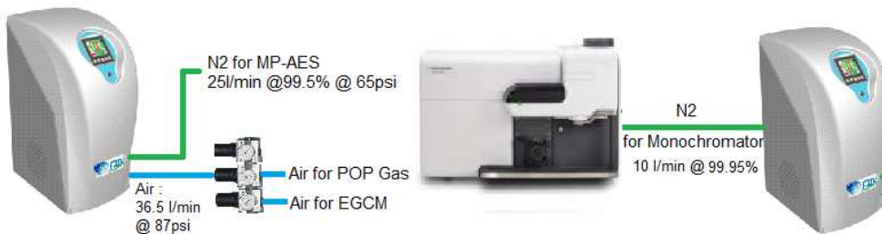
Configuration to purge the monochromator with N 2 to allow determination of sulfur :
