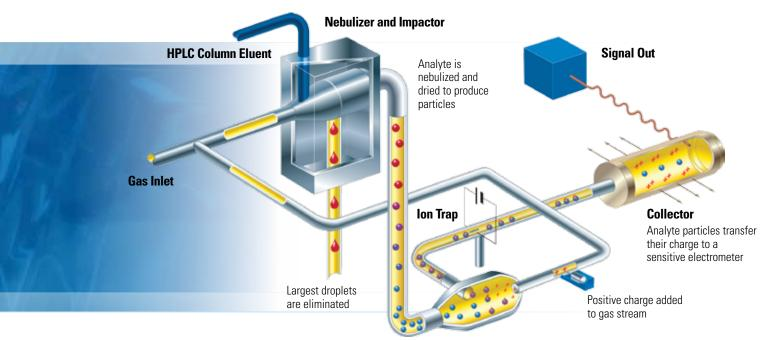
Positive charge is transferred to analyte particles
