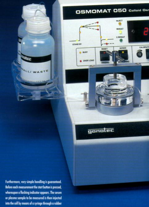
The cell is adequately rinsed with sample solution, if approx. 50 µl portions, from a syringe of 250 µl capacity, are injected in three separate steps at short
