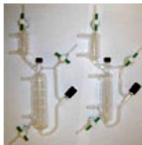
Designed for measurement of larger volume samples (> 100 mL), the Large Volume Purge System has about twice the volume of the original purge system and permits measurements of nanomolar levels of NO and its reaction products without the need to frequently change the reagent. Current users of the original purge system can upgrade to the larger volume system by purchasing the large purge vessel glassware only (CASM 03293-01).
